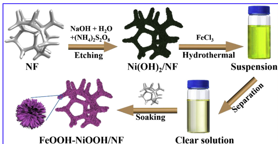
Scheme 1 – Schematic illustration of the synthesis process for FeOOH–NiOOH/NF.
